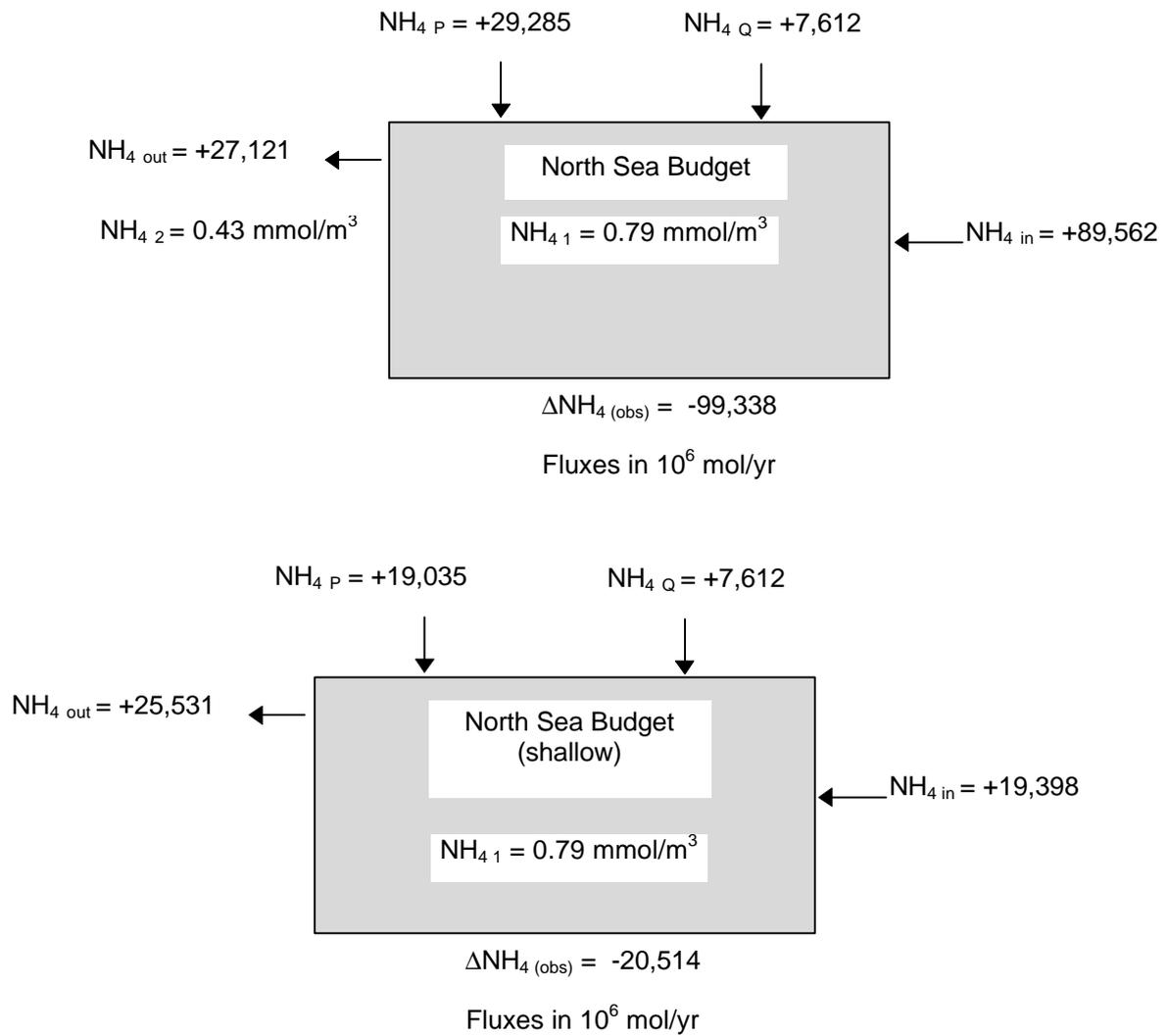
Figure 11.  $\text{NH}_4$  budget for the whole North Sea (top) and for the shallow North Sea excluding the Skagerrak (bottom).
